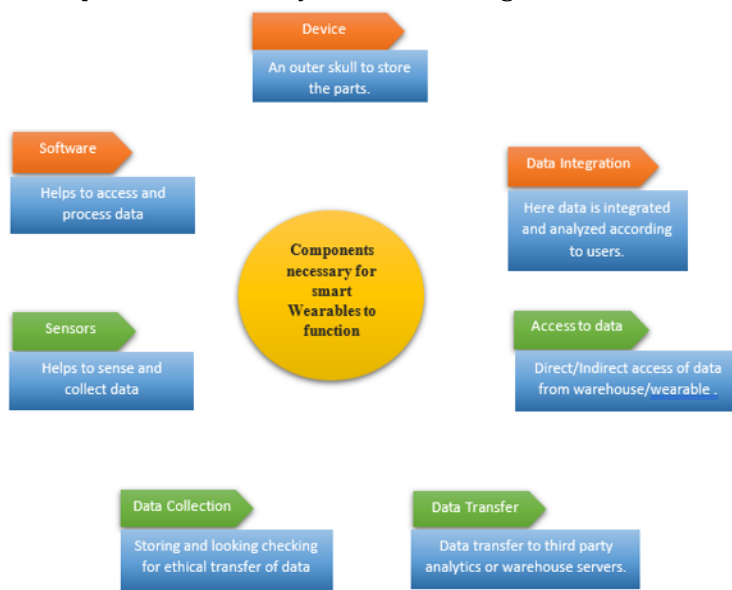
Figure 4: Components necessary for the working of smart health wearable.
